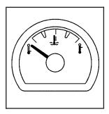
This gage displays the temperature of the vehicle's engine.
